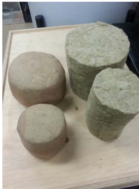
Figure 2: Compressed and uncompressed porous materials.
