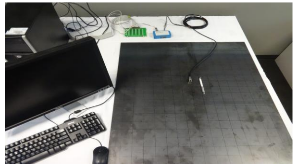
Figure (3) The experimental set-up for the steel plate
