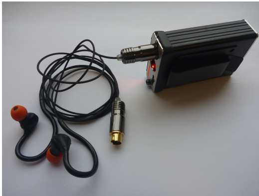
Figure 1: Overview of Auditory Research Platform, as a pair of instrumented earplugs (here equipped with a generic eartip) and a belt-pack processing unit.
