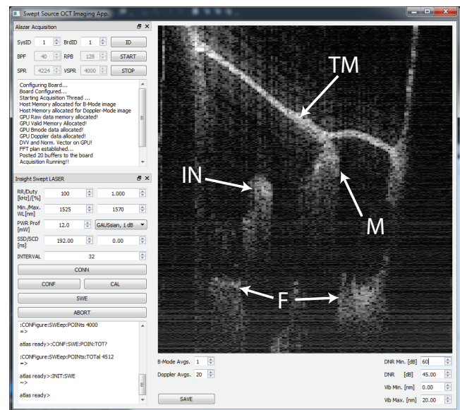
Figure 2: Screen capture from the real-time imaging GUI during in vivo imaging. The entire tympanic membrane (TM), the malleus handle (M), the end of the long process of the incus (I), and the floor of the middle ear (F) are all captured in the same image acquired down the intact ear canal
