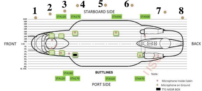
Figure 1: CH-147F Measurement Locations [3]
