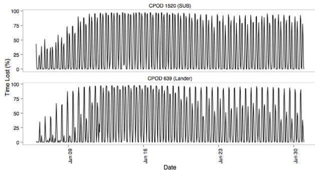
**Figure 3:** C-POD percent-lost time plots. Top: SUB Buoy mounted C-POD 1520; Bottom: platform mounted C-POD 639. The series of peaks represent the sequence of flood and ebb tides with flood tides showing greater % lost time compared to ebb tides. A spring neap pattern is also evident.
