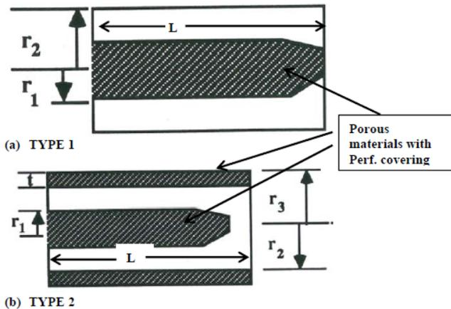
Figure 1: Schematic details of annular silencers.
