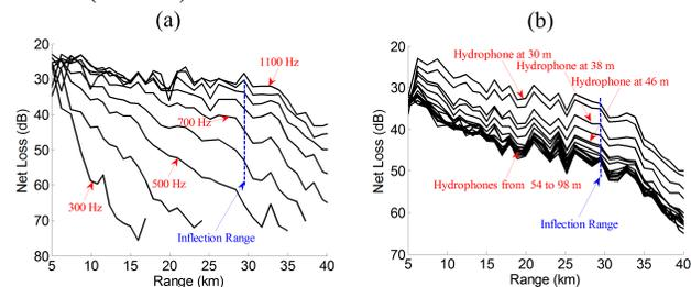
**Figure 1:** (a) Transmission loss versus range compensating for the cylindrical spreading loss (net loss) at the depth of 30 m. (b) Comparison between the net losses at 900 Hz of all the 18 hydrophones.
