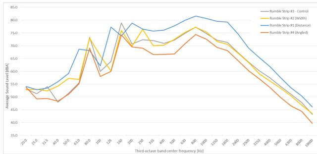
**Figure 4 - Rumble Strip Change in Frequency Spectra**
