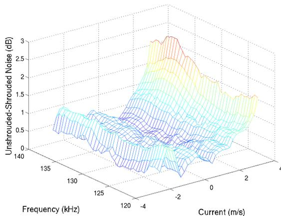
**Figure 4:** The difference in mean ambient noise (dB re  $1\mu\text{Pa}^2/\text{Hz}$ ) between shrouded and non-shrouded icListenHF hydrophones. Note that the difference is low overall (mostly  $< 1$  dB) and greatest at depth averaged speeds  $> 3$  m/s on the flood tide.
