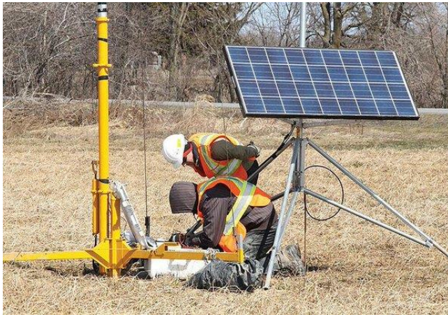
Figure 1 On site noise measurement system
