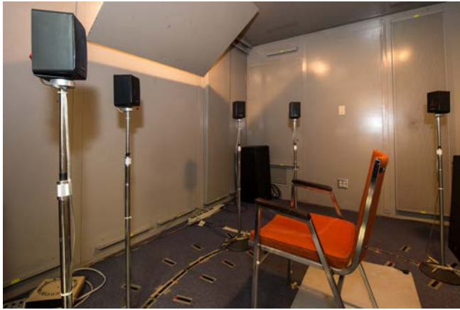
Figure 2: Sound localization set up in the Hearing Research Laboratory. Photo credit: Jim Clark.
