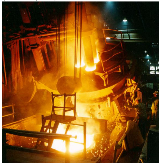
Figure 2. Electric Arc Furnace - Typically >110 dBA @ 10m
