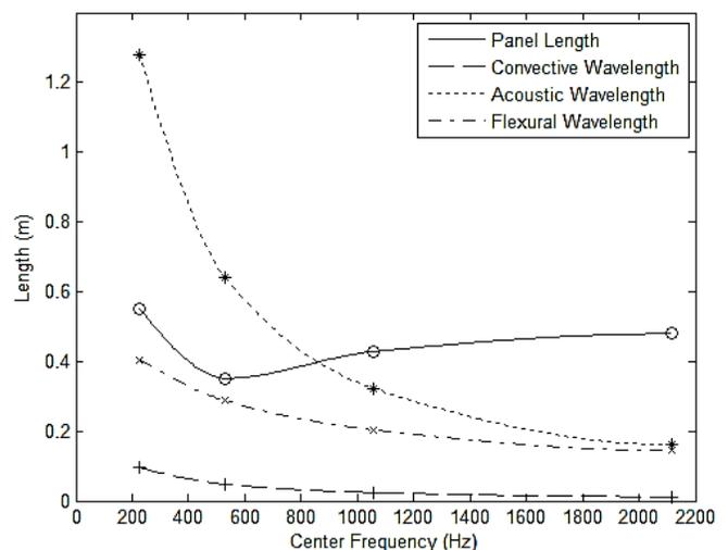
**Figure 5:** Optimal panel length at the center frequency of different octave bands that result in a local minimum average acceleration PSD compared to the calculated flexural wavelength, convective wavelength and acoustic wavelength.
