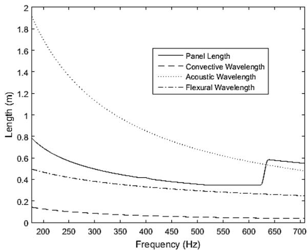
**Figure 6:** Optimal panel length at individual frequencies that result in a global minimum average acceleration PSD compared to the calculated flexural wavelength, convective wavelength and acoustic wavelength for two octave bands.
