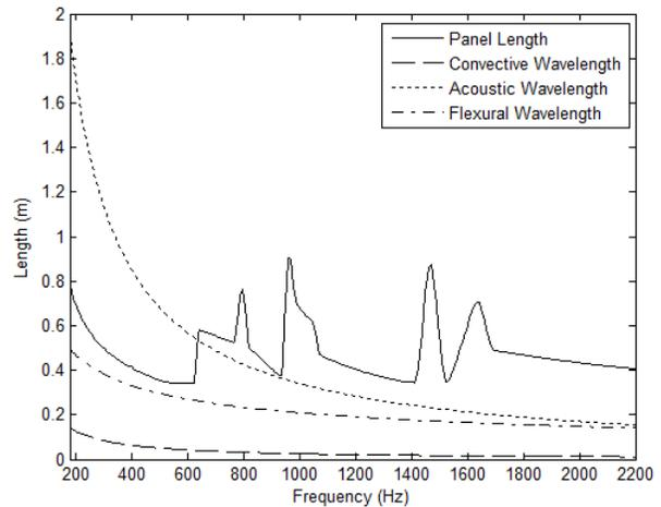
**Figure 7:** Optimal panel length at individual frequencies that result in a global minimum average acceleration PSD compared to the calculated flexural wavelength, convective wavelength and acoustic wavelength for four octave bands.
