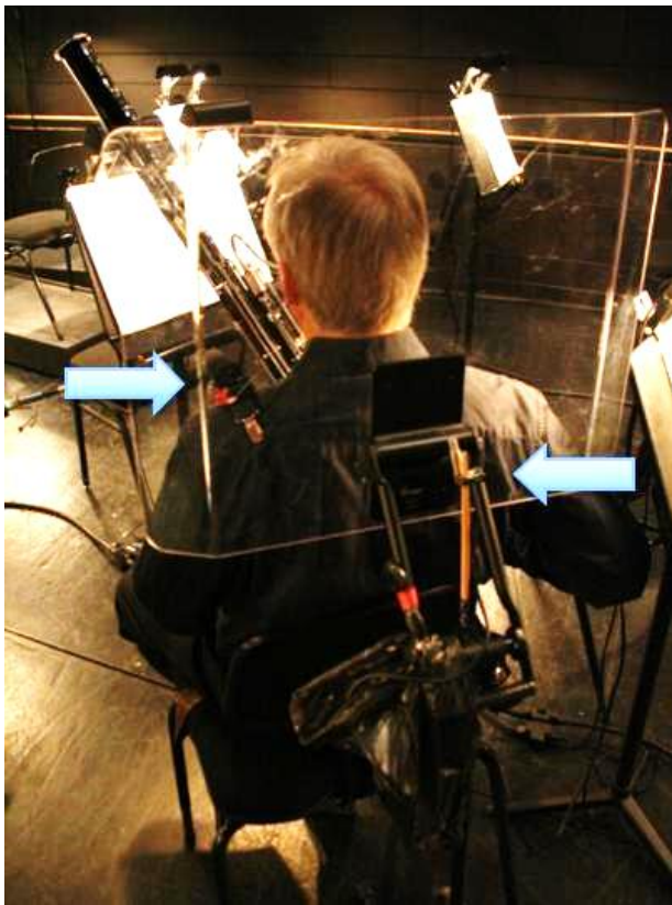
Figure 1: Photo of the dosimeter setup. The arrows in the photo point out the locations of the personal and area dosimeter.
