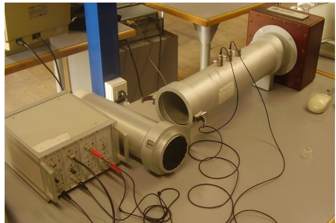
Figure 9. Impedance tube (tube of Kundt) used for the sound absorption coefficient measurements
