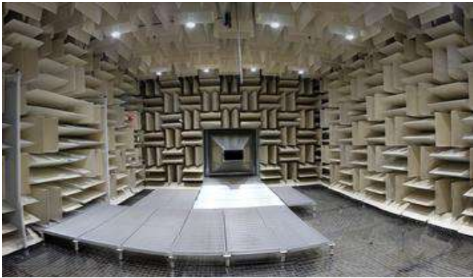
Anechoic room and wind-tunnel opening at GAUS
