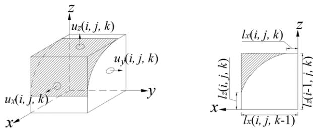
**Figure 1:** 3D conformal mesh and its projection. Left is a conformal grid cell and right is its projection on the  $xoz$  plane.
