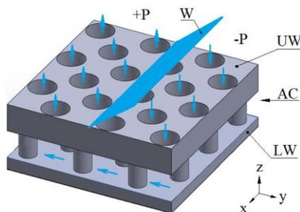
AC – air cavity; W – sound wave; UW – upper wall;
