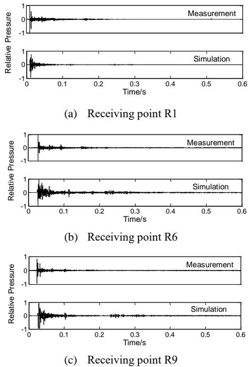
**Figure 5:** The measured and simulated impulse responses of three receiving points.
