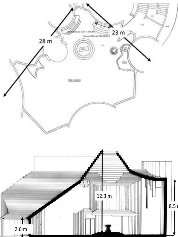
Figure 1: Plant and Section of the church.
