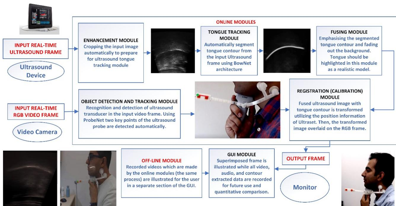
**Figure 9:** The detailed architecture of our multimodal, real-time, and automatic ultrasound-enhanced pronunciation training system comprises of two main online and offline modules.
