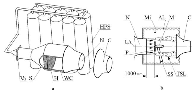
AL – Acoustic lining; P – propeller; Mi – microphone;
