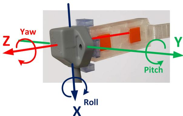
**Figure 12:** Tracking magnetic sensor was attached on UltraChin. Arrows show 6 degree of freedoms defined in our experiments.
