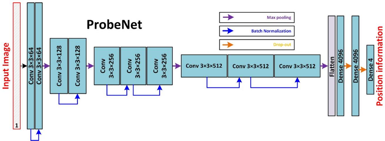
**Figure 7:** ProbeNet architecture for tracking landmarks on the UltraChin. Output layer provides two sets of numbers as vertical and horizontal positions of each landmark.
