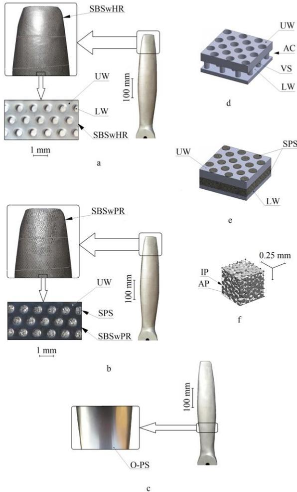
**SBSwHR:** UW - upper metal wall; AC - air cavity;
