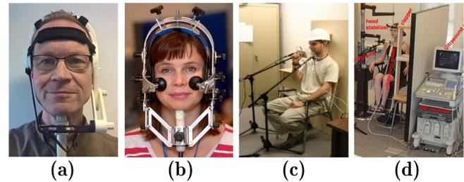
**Figure 4:** An illustration of some stabilization methods for head and probe. Designed helmets keep the probe under the chin, a) [34] b) [35]. One helmet which is fixed to the wall [36], and d) Optical tracking system for the head alignment [22].
