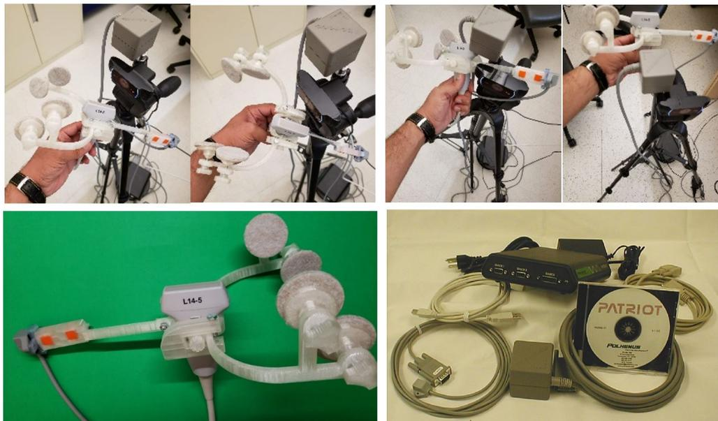
**Figure 11:** First row : different views of magnetic tracking sensors attached on UltraChin. Second row : Different parts of UltraChin and magnetic tracking sensor can be seen in figure.
