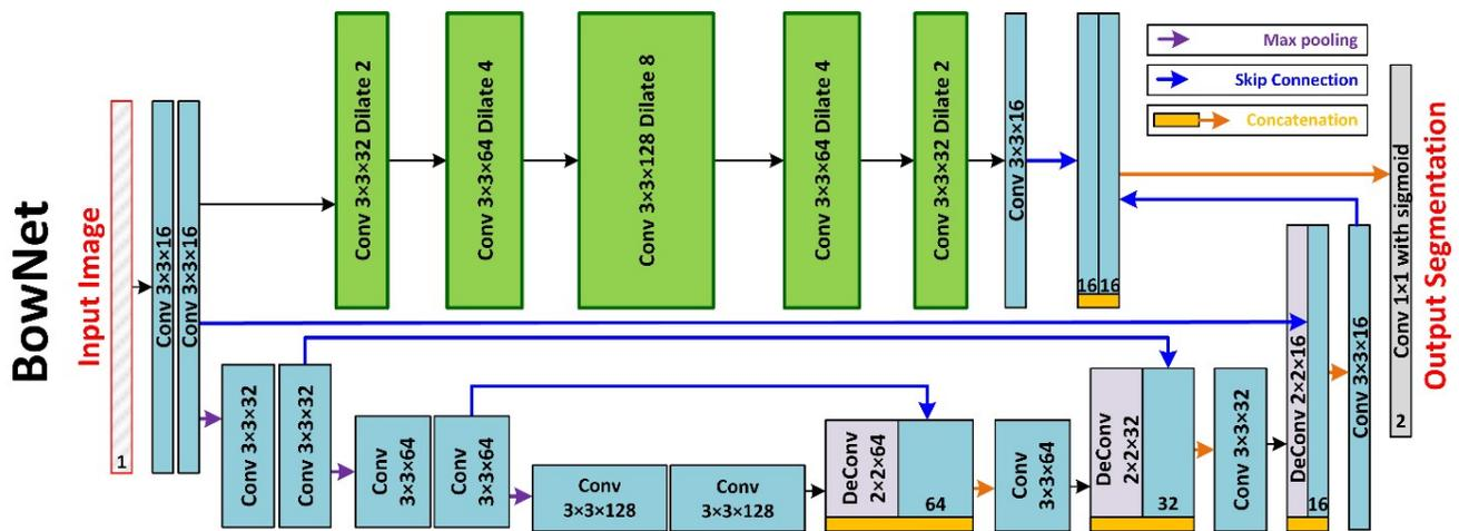
Figure 8: BowNet network architecture for tongue contour extraction automatically and in real-time [48]
