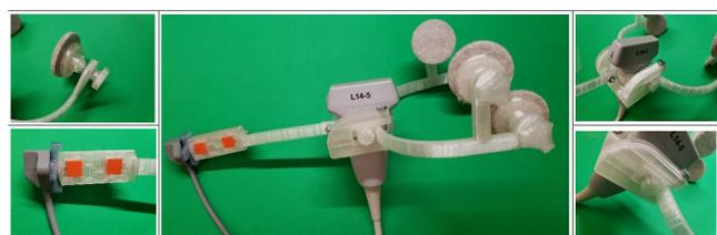
**Figure 6:** The last generation of UltraChin comprises of several modules. This version is universal and usable for different ultrasound probes as well as capable of being attached to other sensors.
