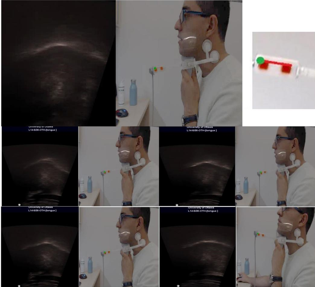
**Figure 13:** Sample frames of our real-time multimodal system. Thick white lines on the right-side images are extracted tongue contours from the corresponding left-side ultrasound images. Red line between two markers is illustrated as a guide.
