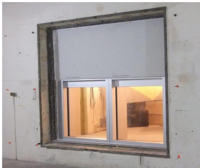
Figure 2 : Window Specimen prepared for STC-testing, showing Filler Wall above Specimen
