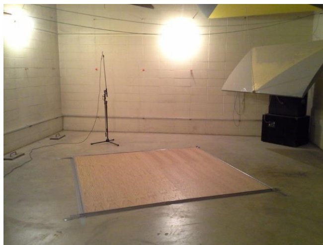
Figure 1: Specimen prepared for ASTM C423 testing.
