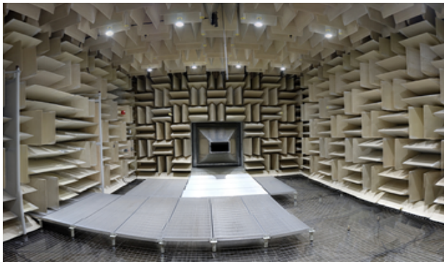
Anechoic room and wind-tunnel opening at GAUS
