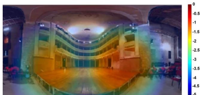
Figure 15: Example of a graphical analysis showing strong reflections hitting the sidewalls of the proscenium. The scale of values represents the difference in intensity, not the absolute values.
