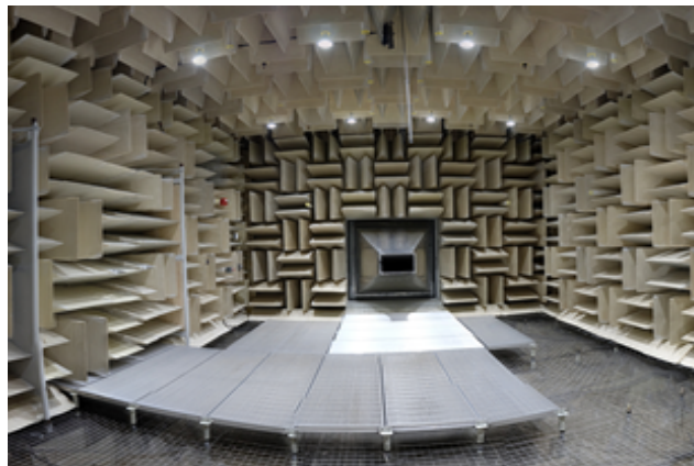
Anechoic room and wind-tunnel opening at GAUS
