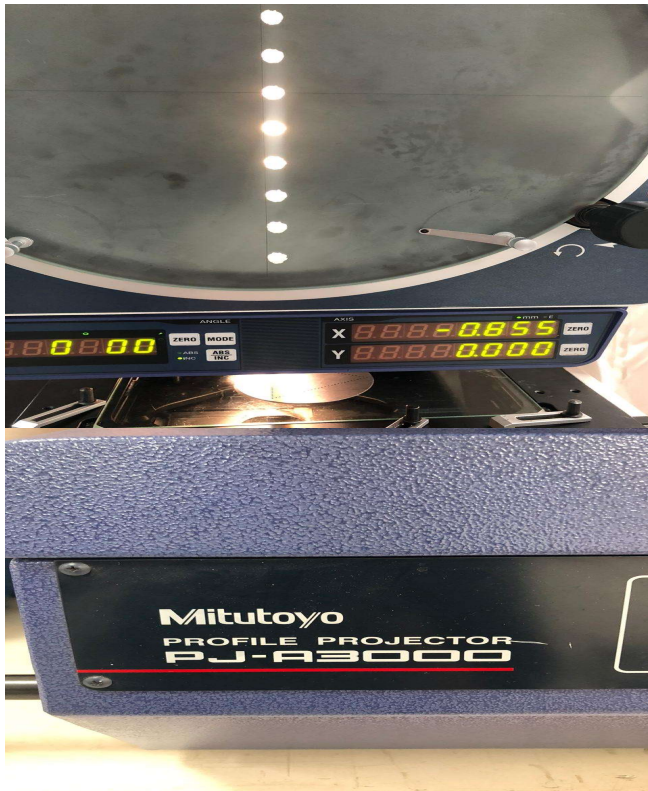
Figure 6: Profile projector image of laser drilled perforations in imperfect circular shapes.
