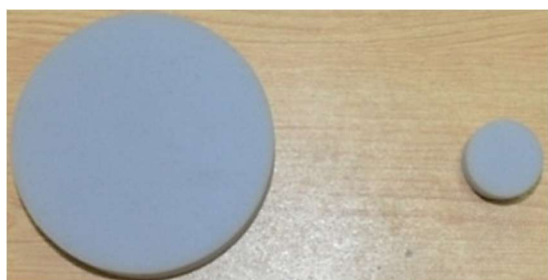
Figure 5: Testing samples of melamine foam (100 mm & 30 mm diameters)
