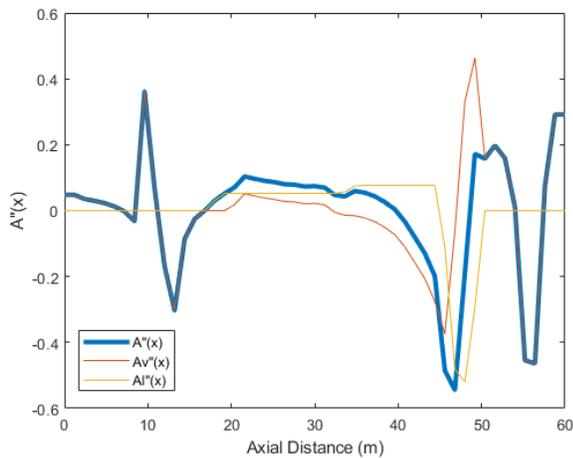
**Figure 6:** Total second derivative function of the SSA ( $A''(x)$ ) combining area displaced by volume ( $Av''(x)$ ) and lift ( $Al''(x)$ )
