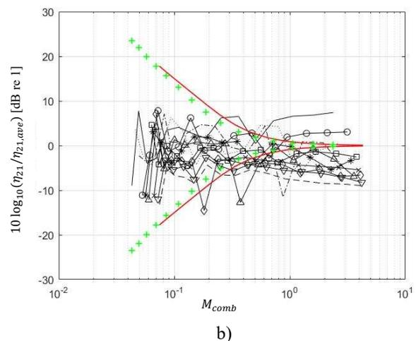
**Figure 3:** Variation of CLF ratio with combined modal overlap factor  $M_{comb}$  for different values of width ratio ( $L_{z2}/L_{z1}$ ) compared to the average over all of the width variations.
