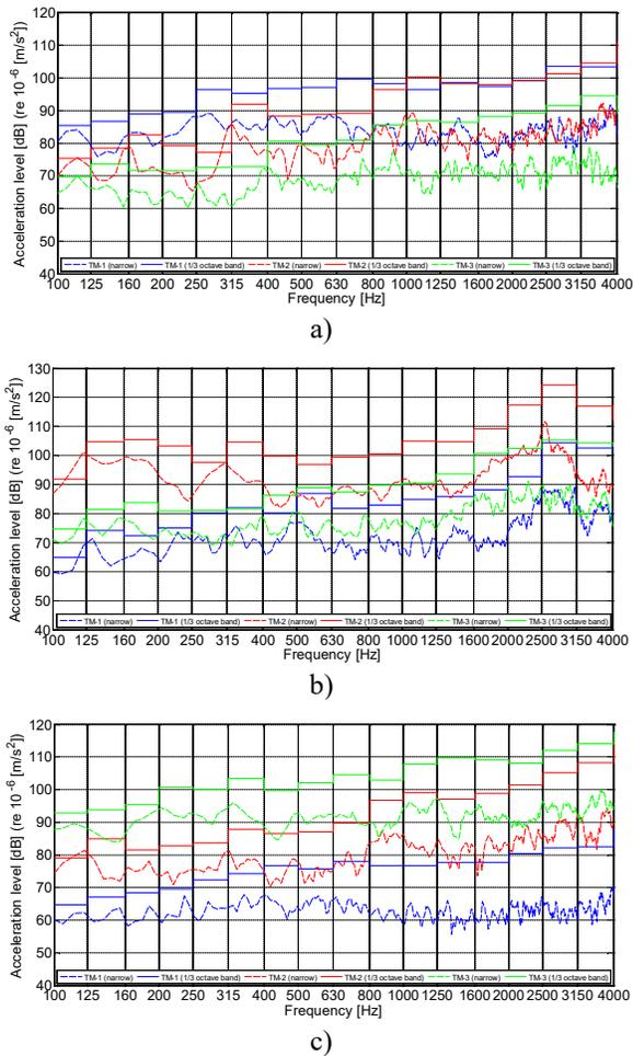
**Figure 5:** Variation of floor acceleration level measured at distinct points considering the tapping machine location. a) point P-1 (living room ceiling); b) point P-3 (bathroom ceiling); c) point P-5 (bedroom ceiling).
