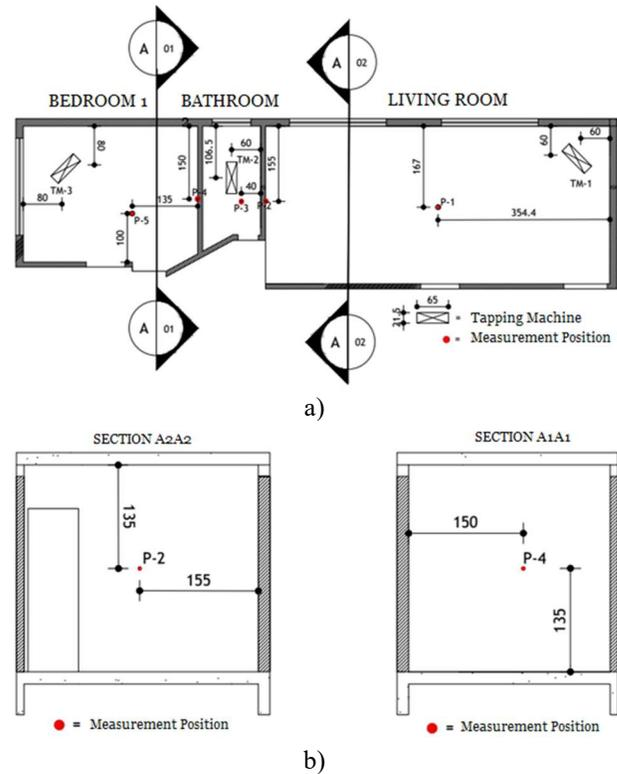
**Figure 3:** Accelerometer and tapping machine positions on the apartment floor (P-1, P-3 and P-5) and walls (P-2 and P-4). a) Floor plan; b) Floor plan cuts (A<sub>1</sub> and A<sub>2</sub>).
