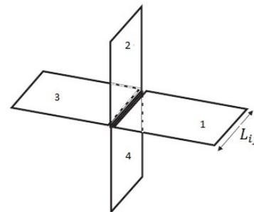
**Figure 4:** Cross-junction type considered for the determination of the vibration reduction index  $K_{ij}$  between floors and walls. The subscripts  $i, j$  represent the source and receiver plate respectively.
