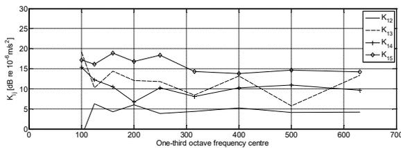
**Figure 8:** Variation of the Vibration Reduction Index ( $K_{ij}$ ) with frequency and accelerometer positions P-1 – P-5. Four different situations were considered:  $K_{12}$  (TM1 – P-2),  $K_{13}$  (TM1 – P-3),  $K_{14}$  (TM1 – P-4) and  $K_{15}$  (TM1 – P-5).
