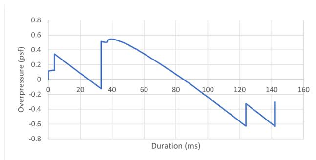
**Figure 9:** Sonic boom ground signature of the SSA propagated using PC Boom with near-field overpressure input (step size of 1.2 m)
