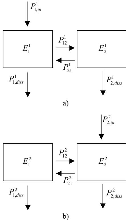
**Figure 1:** SEA models of two rooms separated by a single-leaf partition approximated by a two-subsystem model. Therefore, only the non-resonant transmission path is considered. a) Power is injected into subsystem 1; b) Power is injected into subsystem 2. The subscripts ‘i j’ denote the power flow from subsystem ‘i’ to subsystem ‘j’ and the superscript indicates which subsystem is under direct excitation.
