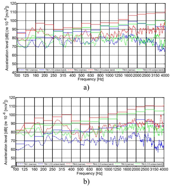
**Figure 6:** Variation of wall acceleration level measured at distinct points considering the tapping machine location. a) accelerometer on point P-2 (living room wall); b) accelerometer on point P-4 (bedroom wall).
