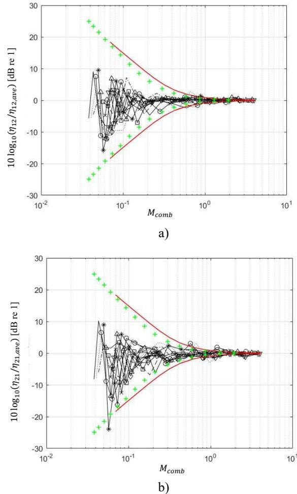
**Figure 2:** Variation of CLF ratio with the combined modal overlap factor  $M_{comb}$  for different values of height ratio ( $L_{y2}/L_{y1}$ ) compared to the average over all of the height variations.
