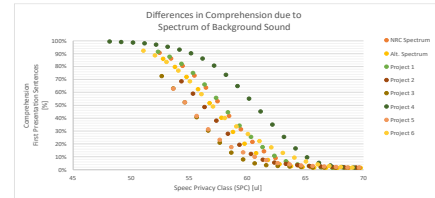
Figure 4: The relationship between SFP comprehension and SPC, for each spectrum, for a range of DL conditions.
