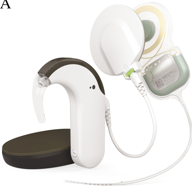
FIGURE 11 – A : external and internal components of the MED-EL SYNCRONY 2 cochlear implant system (image courtesy of MED-EL). B : CI's external components can be tailored specially for children, as the Sky CI™ M sound processor designed for kids by Advanced Bionics (image courtesy of Advanced Bionics).
