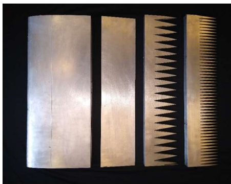
Figure 8: From left to right: NACA0012 main body, TE of case E0, TE of case E1 and TE of case E2.
