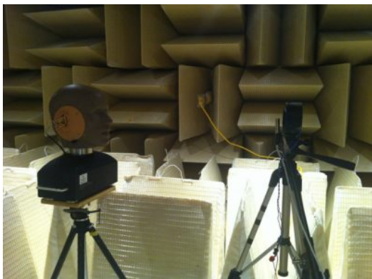
Figure 3: Test set-up in the anechoic room
